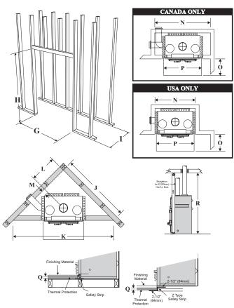
NOTE: Safety strip is required when the fireplace rests on a combustible surface, and should extend 2" in front and on the sides of the fireplace. When using a wooden support to raise the fireplace. A "Z" type safety strip, not supplied, must be fabricated (Use 20 gauge galvanized sheet steel).
